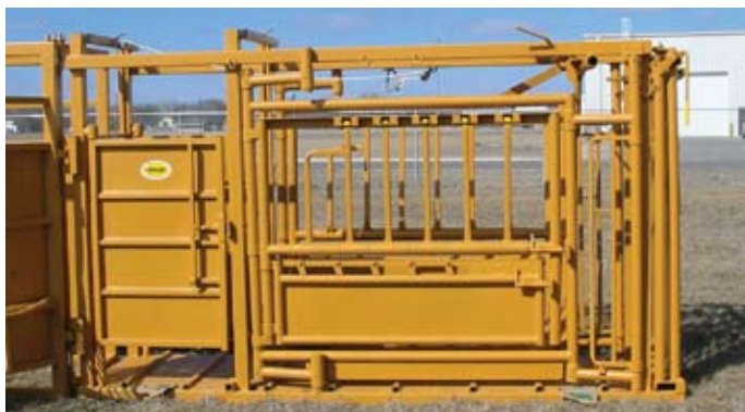
Straight wall squeeze. Attached palpation cage. Drop bars open individually. Steel floor. Automatic headgate.
