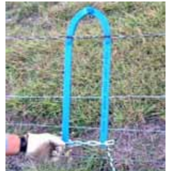
Step 6. Loosen the chain and remove tool from wire.
