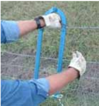
Step 3. Lay a short length of spare wire across face of tool.
