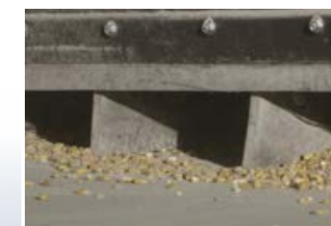
Flexible Rubber Paddles Move Grain Gently To Sump.
