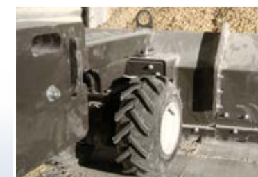
Tires Are Foam Filled, With Tractor Tread.
