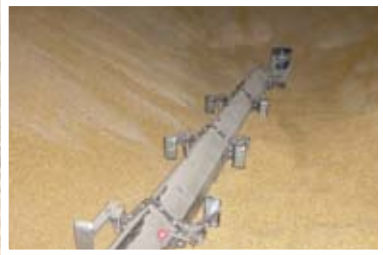
Design allows Sweep to follow contour of floor.
