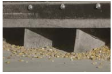
Moves grain gently and evenly to sump with flexible rubber paddles.
