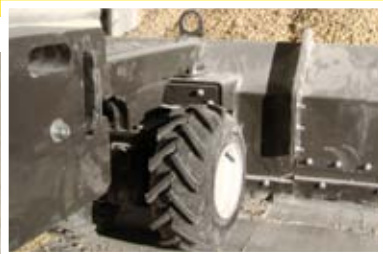
Tires are foam filled, with a tractor tread. Drive tire size is 13 x 5.00-6 Super Lug.
